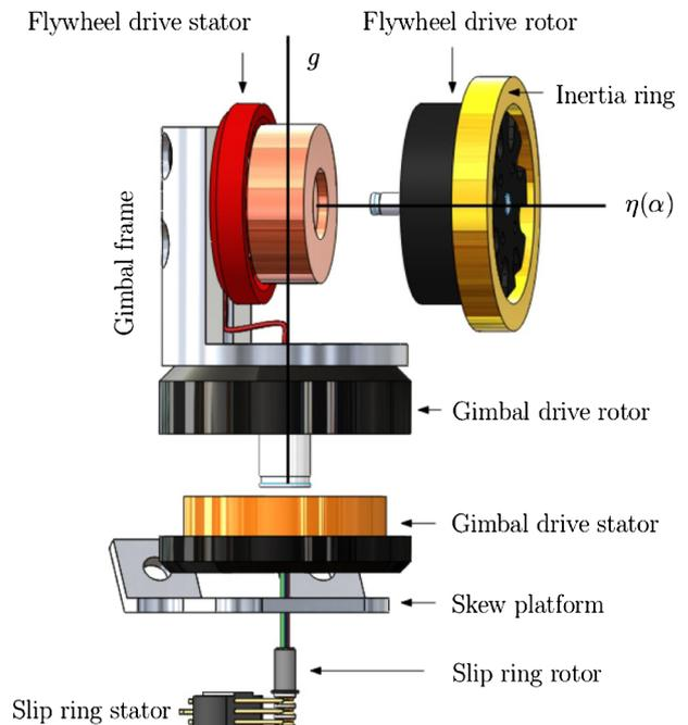
Fig. 3 Exploded view of ASCMG showing functional components.
