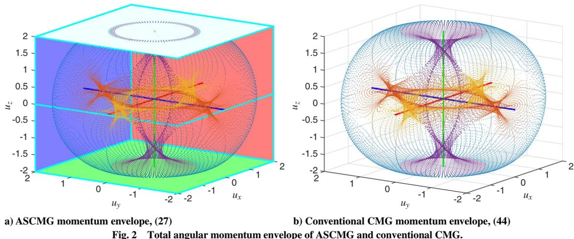
Fig. 2 Total angular momentum envelope of ASCMG and conventional CMG.
