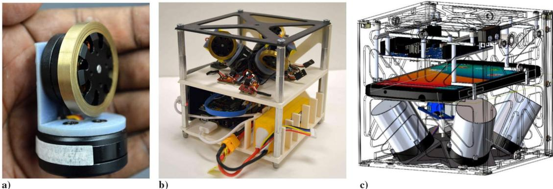
Fig. 4 Representations of a) unit ASCMG prototype, b) prototype of three-ASCMG cluster in 1U cubesat, and c) four-ASCMG pyramid cluster.
