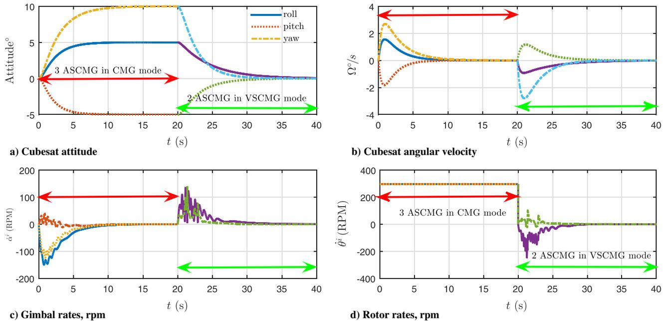
Fig. 5 Numerical simulation results of an agile 1U cubesat with three ASCMGs.
