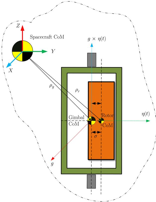
**Fig. 1** Schematic of ASCMG showing an offset  $\sigma$  between the rotor and gimbal center of mass.
